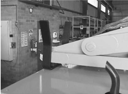
Ensure the light bar is stowed in towards the mast and is locked against the stop prior to towing.
