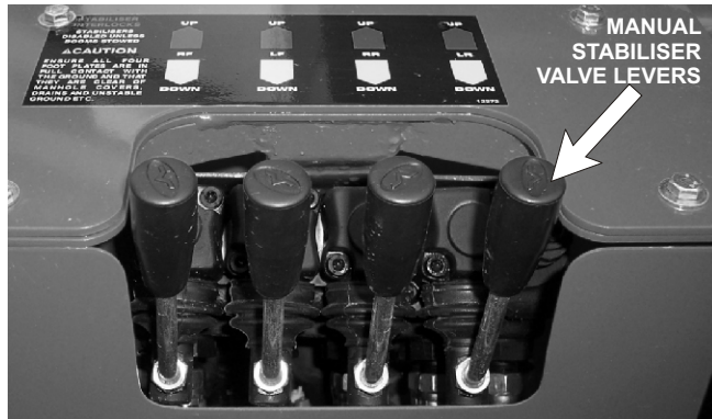
Figure 6.7 - Stabiliser Controls (Manual)
