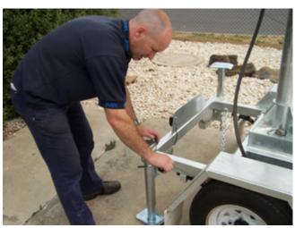
3. **Undo the Mast Brake**. This is important! Once the Mast Brake is undone, you can then swivel the Sign head left or right so that the message can be easily read by passing traffic.
