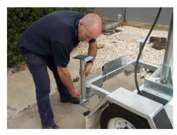
2. Pull out the Pin that holds each of the Stabilization Legs into place, and then reinsert the Pin once the Leg has been swung out. You can then wind the Leg up or down so that the angle of the Sign head is correct, and to ensure Sign stability in windy conditions.
