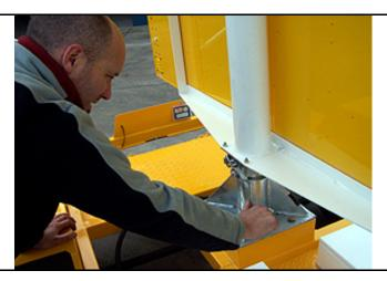
4. Use the Switch located in one of the battery boxes to raise the Sign head to an appropriate level. Then lock the Mast Brake to hold the Sign in position.
