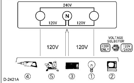
ii) **120V / 240V** - Voltage selector in 120V/240V position
