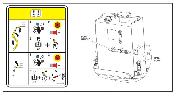
Figure 5-1. Auxiliary Descent Decal and Hand Pump
