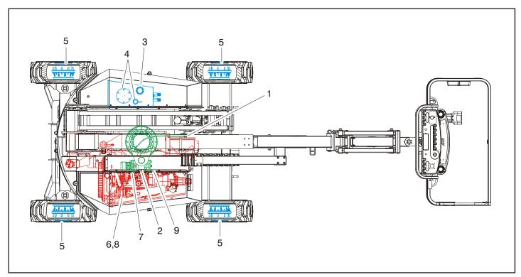
Figure 6-6. Operator Maintenance and Lubrication Diagram
