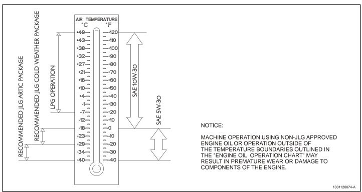
Figure 6-4. Engine Oil Operation Chart - GM
