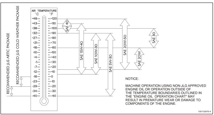
Figure 6-5. Engine Oil Operation Chart - Kubota
