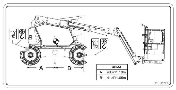
Figure 4-6. Lifting and Tie Down Chart
