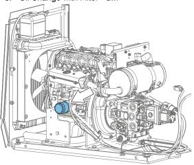
Lube Point(s) - Fill Cap/Spin-on Element Capacity - 3.1 Quarts (3 L) w/Filter Lube - EO
