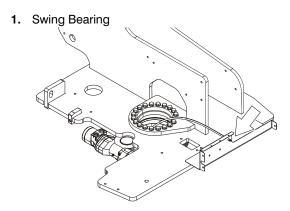
Lube Point(s) - Remote Fitting Capacity - A/R
