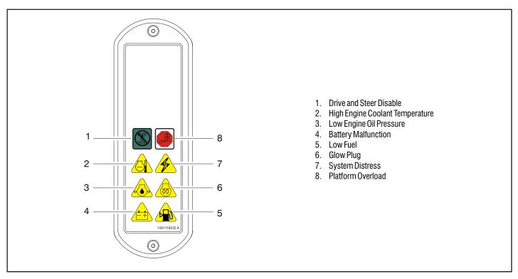
Figure 3-2. Ground Control Indicator Panel
