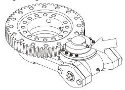
Lube Point(s) - Grease Fitting Capacity - A/R Lube - BG Interval - A/R
