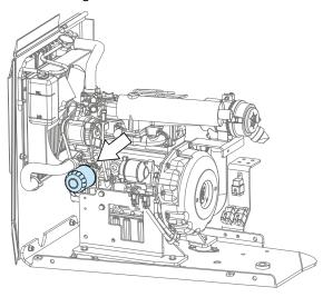
Lube Point(s) - Fill Cap/Spin-on Element Capacity - 5.4 Quarts (5.1 L) w/Filter Lube - EO
