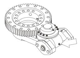
Lube Point(s) - Grease Fitting Capacity - A/R Lube - Mobile SHC 007 Interval - A/R
