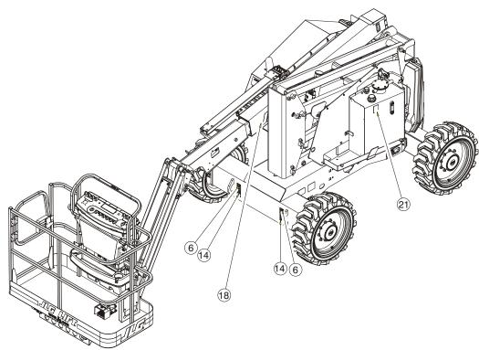
Figure 4-7. Decal Location Sheet 1 of 10
