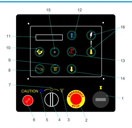
Figure 6-1 Ground controller (DTC system)
