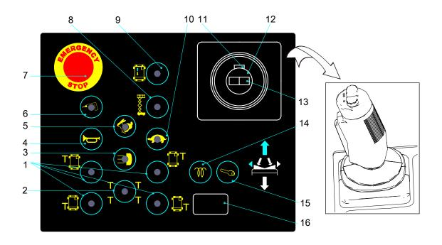
Figure 6-5 Platform controller (DTC system)
