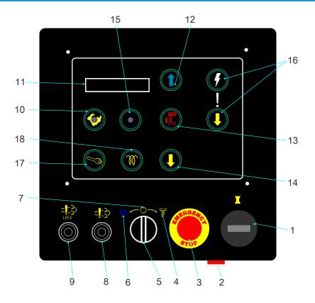
Figure 6-2 Ground controller (DTC system)-for EU Stage 5 engines
