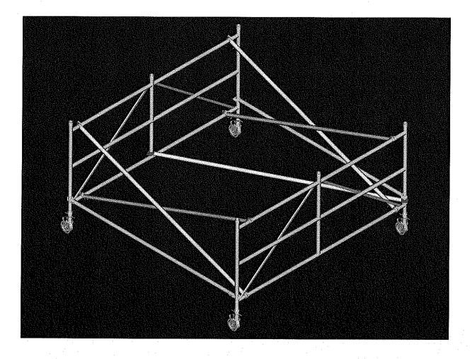
Add upper frames 1.9m high, 1.4m high and 0.9m high as required, installing 4 diagonal braces per lift in 1.3m wide gear. Each brace should be attached to the top transom of the frame below and as near as practical towards the outside of the frame.
