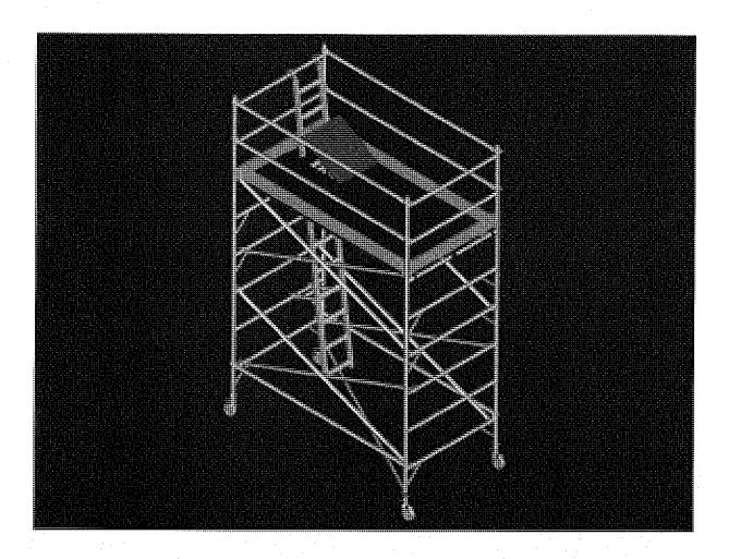
Please note that when horizontals are clipped to standards (vertical component) they are designed for sideways deflection only and are not load supporting. Therefore do not step on these horizontals when climbing the scaffold. Do not stand on midrails and handrails.
