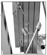
The winch handles have been placed in the stored position.
