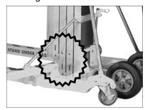
Pull the tool down and the brake will release.
