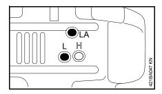
Adjust idle speed with the idle speed screw (LA) so that the drilling spindle does not rotate.
