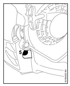
Press the manual fuel pump bulb (5) at least five times.
