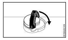
Fold the grip flush with the top of the cap.
