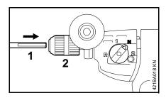
Insert the drilling tool (1) in the chuck (2) and tighten it firmly.
