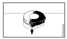
The lug on the grip must fully engage the recess (arrow).
