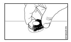
Grip the cap – it is properly locked if it cannot be turned or removed.
