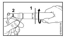
Hold the handle (1) by the clamp and turn it clockwise until the gap (2) is completely closed.
