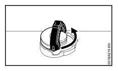
Rotate the tank cap about a quarter turn counterclockwise.
