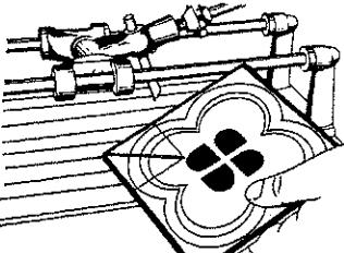
You will have now, on the glazed side, the first two scratches made with the cutting wheel and the vertex to vertex groove.
