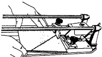
In order to make diagonal cuts, a separation could be made by placing the oblique-shaped piece under the separator.
