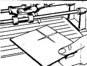
Now, change the scoring wheel by the Punching Tool. Turn the tile and score the bisque marking the square angle until you have two grooves 3-4 mm. deep.
