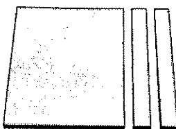
If you want a 2 cm. wide piece, score the tile at 2 and 4 cm. Separate it by the 4 cm. scratch. Finally, separate it by the 2 cm. scratch.
