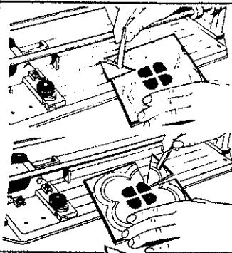
You don't have to use de separator, simply take the tile and hit softly on the glazed side until you separate the two triangles, as you can see in the figures.
