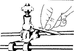
Put the scoring wheel in the ram and fix it with the handle.
