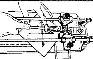
Now, open two more grooves on the bisque from vertex to vertex of the square, all the way down to the glaze.
