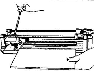
Turn your tile over to the glazed side and using your guide score the glaze using a scoring wheel.
