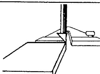
Put the miter in the ram. Place the tile with the bisque face up.
