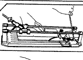
In order to avoid damage to the glaze we recommend to stop mitering when there is only 1 mm. of bisque left.
