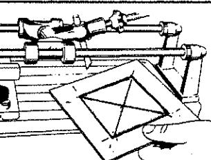
Figure showing the grooves on the bisque. The vertex to vertex grooves have gone through the whole tile.
