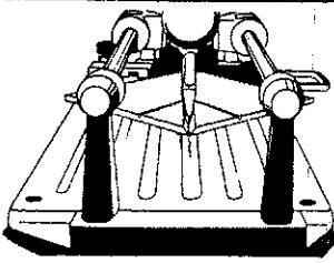
Place the tile in such a way that you can make a diagonal groove all the way down to the glaze, from the vertex of the tile to the vertex of the square angle.
