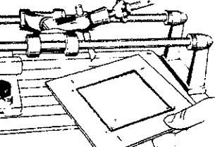
Change the scoring wheel by the Punching tool, and score until you get four grooves 2 - 3 mm. deep following the exact pattern you made on the other side.
