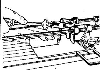
Place the tile on the base (use the support stop for an accurate cut). Score the tile with the scoring wheel only once.
