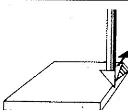
Start mitering on the upper and of the tile in order to give the miter a way out, and being careful not to blunt the tile.
