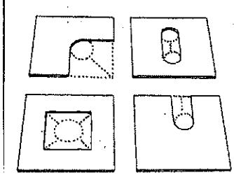
Once you have fixed the drill to the guiding bars of the cutter, all you have to do is turn the crank and drill the bisque, and stop when you arrive to the glaze. You don't have to drill the glaze, simply hit the tile softly on the glazed side and you will have a circle after a few retouches.
