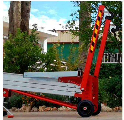
4.- Remove the legs and reinsert them in the base in the vertical position.
