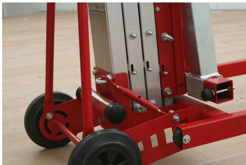
7.- Lastly, put the forks into the horizontal position and secure using the magnetic locking bolts.
