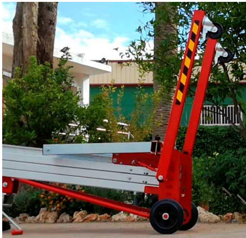
To remove the leg, pull the safety bolt to unblock it, place the leg in the desired position and release the bolt to block them again and secure the position.
