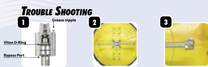
1) If water is leaking from the bypass port in the bottom of the rotary head: Inspect the viton O-Ring in the rotary head.
