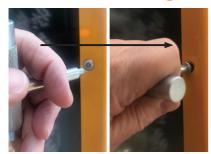
For access to the sign head, use the **"T Tool"** provided in the document pouch under the control box lid
