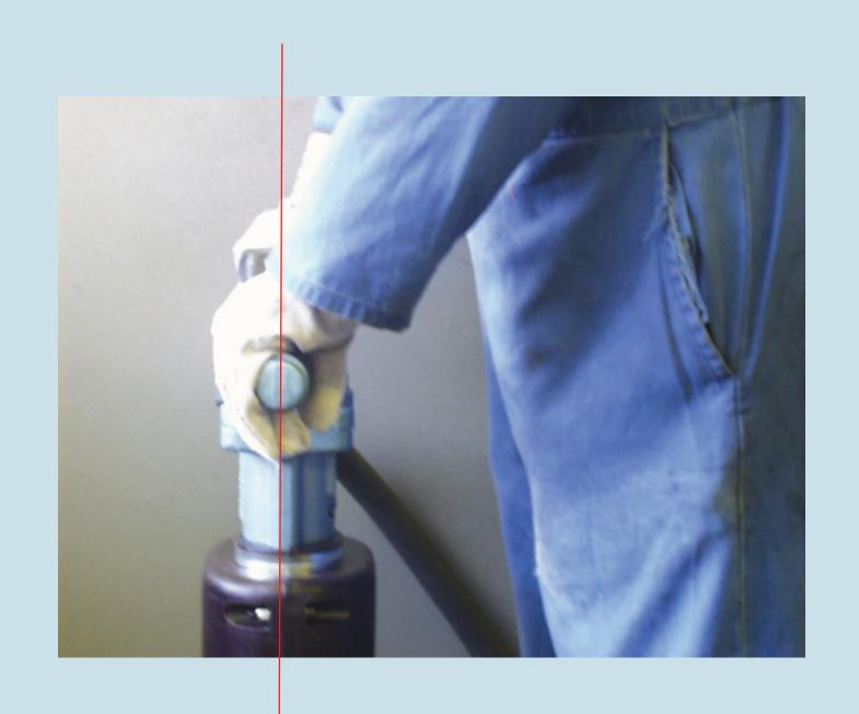
Try to keep the breaker as near vertical as possible during operation.
