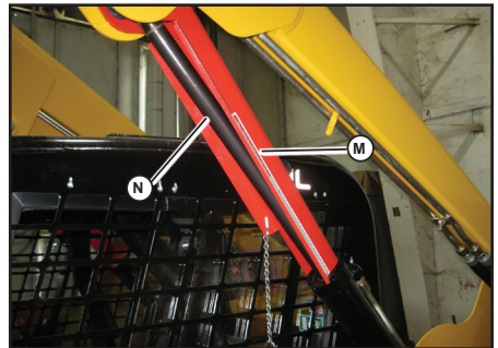
Fig. 29 - Lift Arm Support Applied
